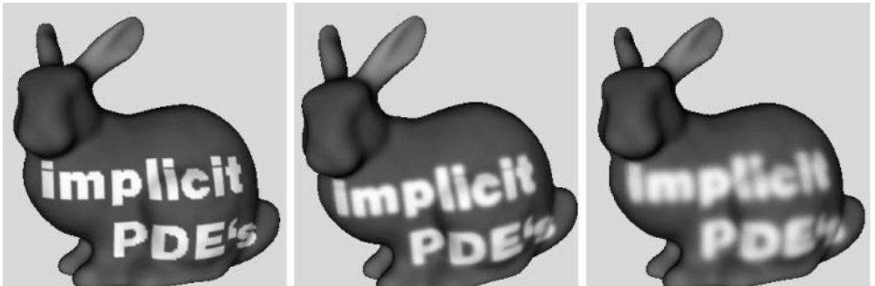
FIG. 1. Intrinsic isotropic diffusion. Left: original image. Middle: after 15 diffusion steps. Right: after 50 diffusion steps.
