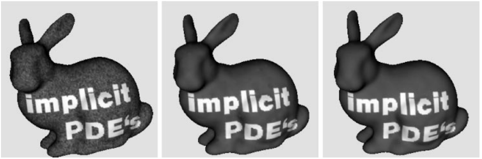
FIG. 2. Intrinsic anisotropic diffusion with constraints (automatic stop term). Left: original noisy image. Middle: after 50 diffusion steps. Right: after 90 diffusion steps. Notice how the diffusion stops and information is not smeared.
